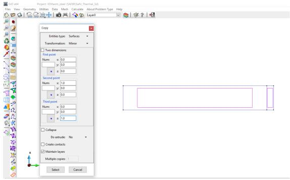
Select the 2 surfaces and press *Finish*. This resulted in the creation of the right half of the lower flange.
