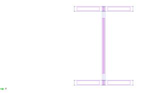
Now, we will extrude this cross section along the length of the profile. Change to the 3d isometric view by selecting from the pull down menu: *View->Rotate->isometric*
