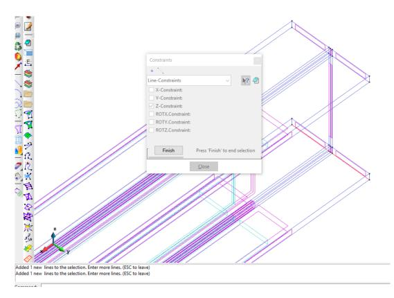
Select Y-Constraint and assign to the section center (vertical) lines at the two ends of the beam. Press [*Esc*].
